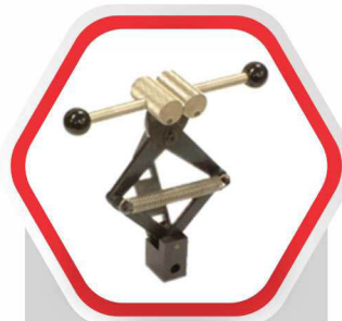
Scissor Grips Scissor grips for flat samples such as foils, plastic film and rubber.
