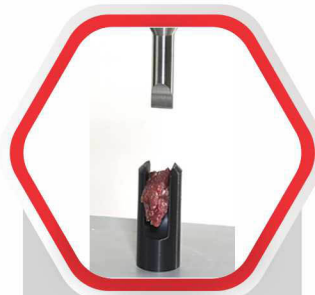
Meat, Poultry and Fish Testing Test the firmness and cutting strength of your meat, poultry or fish.
