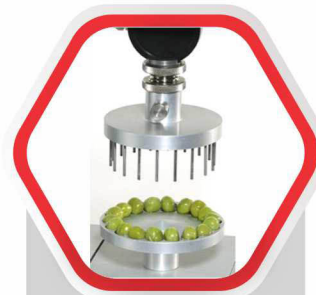
Fruit and Vegetables Testing Test the firmness and extrusion properties on your fruit or vegetables.
